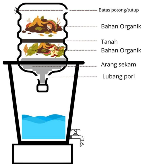
Figure 8. Modified stacking bucket design (Personal Documentation, 2024)
